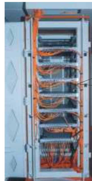
PARAMNet-II Rack interconnecting 64 Compute Nodes of PARAM Padma cluster.
