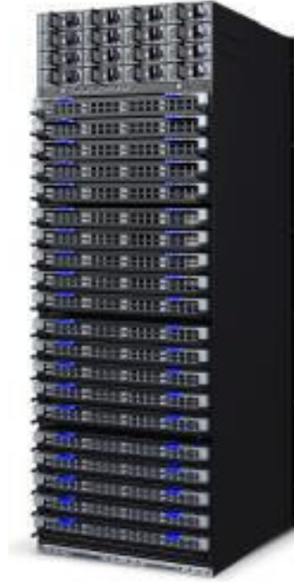
InfiniBand HDR200 Director Switch and IB Cables for Compute Communication
