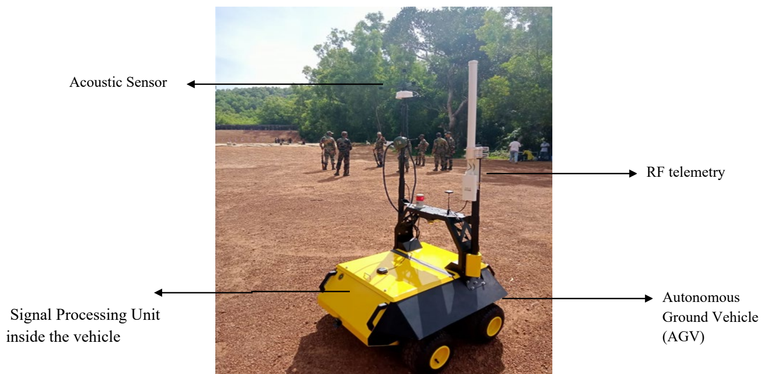
Fig. 2. Vehicle mount system mounted in AGV
