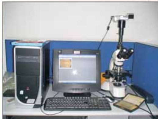
Image capturing setup – Interfacing with microscope and camera
