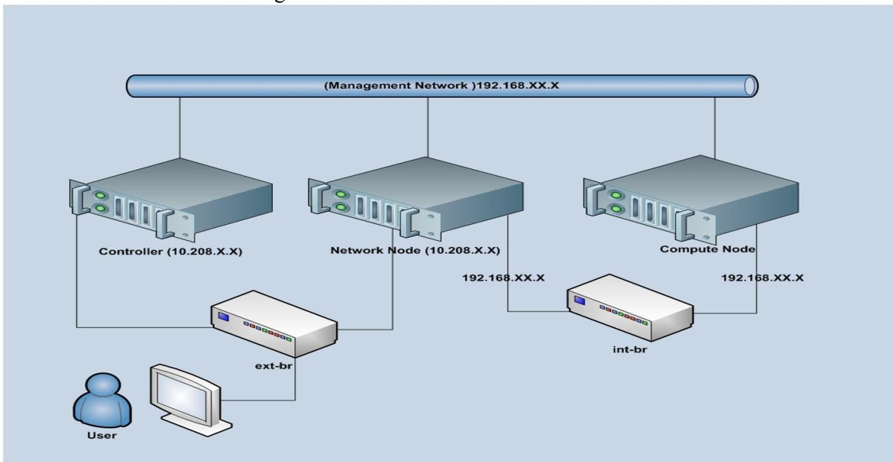
Fig 3. Network Connection between the nodes
